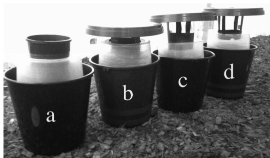
Fig. 2. Evaluation of black lid on the large GAT prototypes on the capture of gravid Ae. aegypti in semifield conditions (experiment 6). (a) GAT as control (no lid); (b) GAT with a 30-cm-diameter black lid (GAT + L) with four entrance windows (7 by 5 cm); (c) GAT with high lid (GAT + HL), the black lid was placed 12 cm above the translucent chamber and four entrance windows (8 by 6 cm); and (d) GAT with high open lid (GAT + HOL) with four entrance windows (12 by 8 cm).
