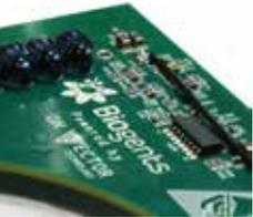
The patented insect sensor consists of arrays of infrared LEDs and light detectors that provide reliable and sensitive detection and differentiation of mosquitoes from other objects entering the trap.
