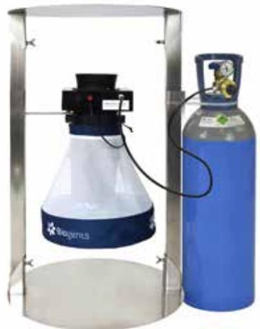
*BG-Counter 2 with a BG-Trap Station and CO<sub>2</sub> source. The station can run on solar power (the solar panel is not displayed here).*
