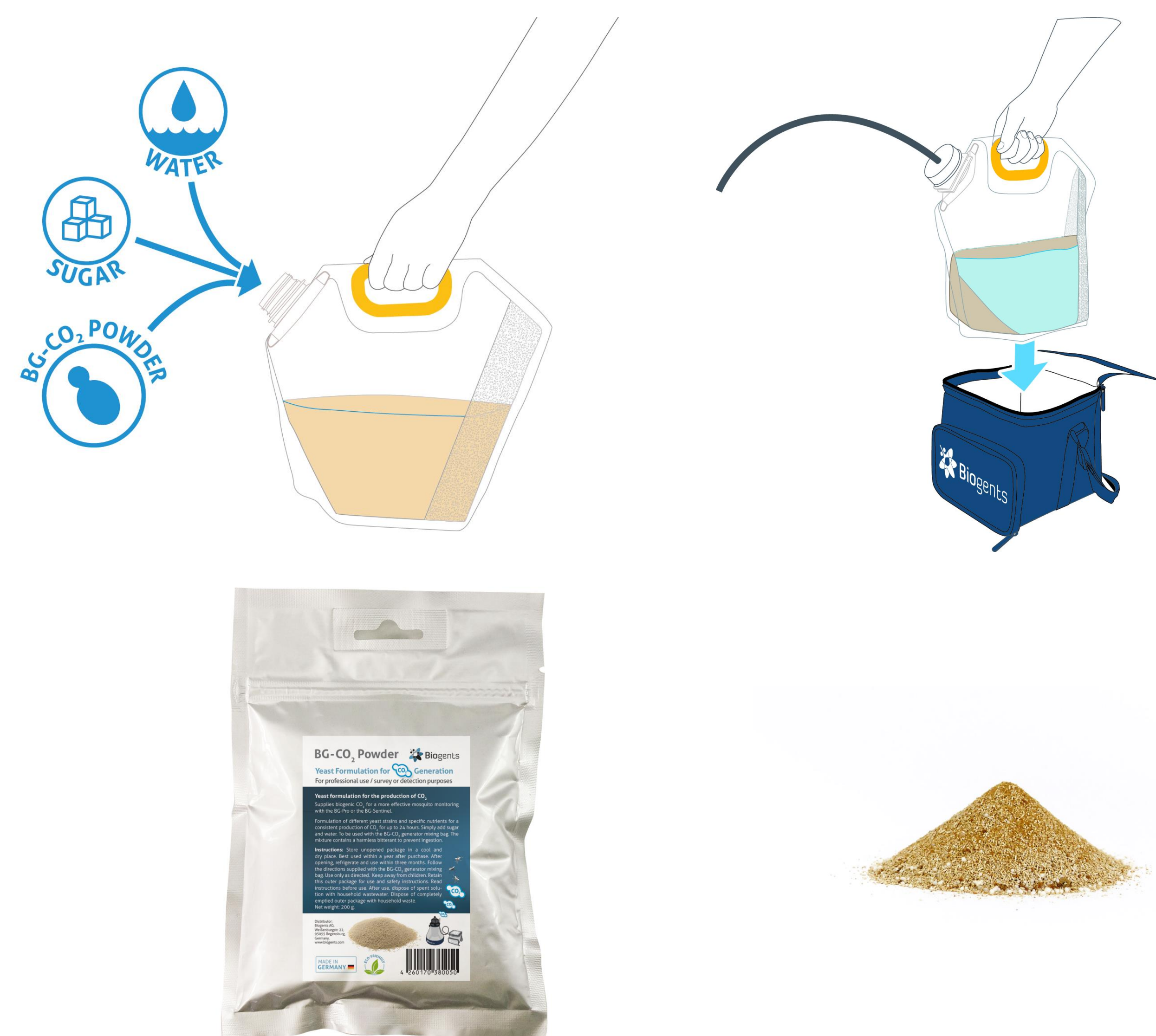
Fig.1 Schematic depiction of the setup of the BG-CO 2 Generator. The culture container is filled with 2 liters of water and 500 g of household sugar and placed inside an insulation bag. The freeze-dried yeast starter culture is available under the brand name "BG-Powder".
