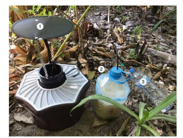
BG-Mosquitaire CO, with rain shield (1), 5 L PET bottle containg 3 L water, 700 g sugar and 40 g yeast (2), and 1.5 L overflow bottle.
